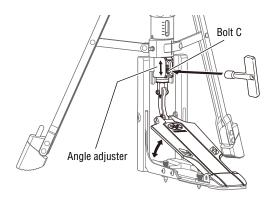
② After the angle has been determined, firmly tighten bolt C with the tuning key.
