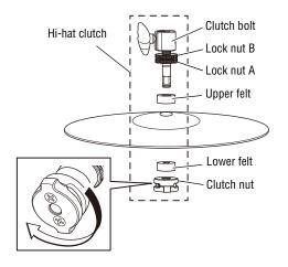
3 Turn the metal part of the clutch nut to the right until it clicks to secure the cymbal. Check that the clutch nut does not fall out. 4 Use the lock nut in order to adjust how tightly the top hi-hat cymbal is gripped. Rotating the lock nut to the right increases tension while turning to the left decreases tension.
