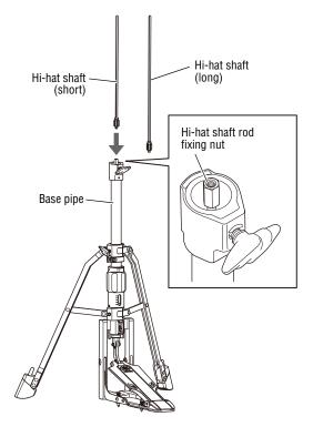
2 Put the hi-hat shaft into the hi-hat shaft rod fixing nut in the base assembly pipe holder to secure it.
