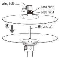
(5) Slide the hi-hat clutch attached to the top cymbal onto the hi-hat shaft, stepping on the footboard to put the desired amount of space between the cymbals, and then tighten the wing bolt.
