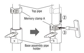
② Loosen the screw of memory clamp A by using a tuning key, and then move the clamp to the boundary line of the top pipe and the base pipe. Also, make sure memory clamp A firmly fits into the hollow on the back of the base assembly pipe holder.
