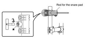
**2.** Lightly screw the clamp bolt into the socket on the snare pad. (Rotate the clamp bolt five to six times.)
