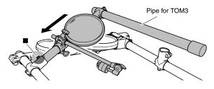
**5.** Tighten the key bolt (■ in the above figure) on the large rack and the clamp bolt of the cymbal holder.
