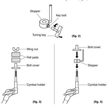
**6.** Place the stopper to make full contact with the bottom surface of the bolt cover and tighten the key bolt with a tuning key to secure the stopper (fig. 5).
