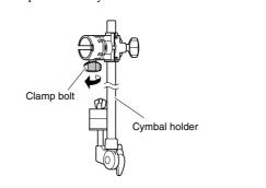
**3.** Slide the holder clamp onto the TOM3 pipe, and lightly tighten the clamp bolt of the cymbal holder.
