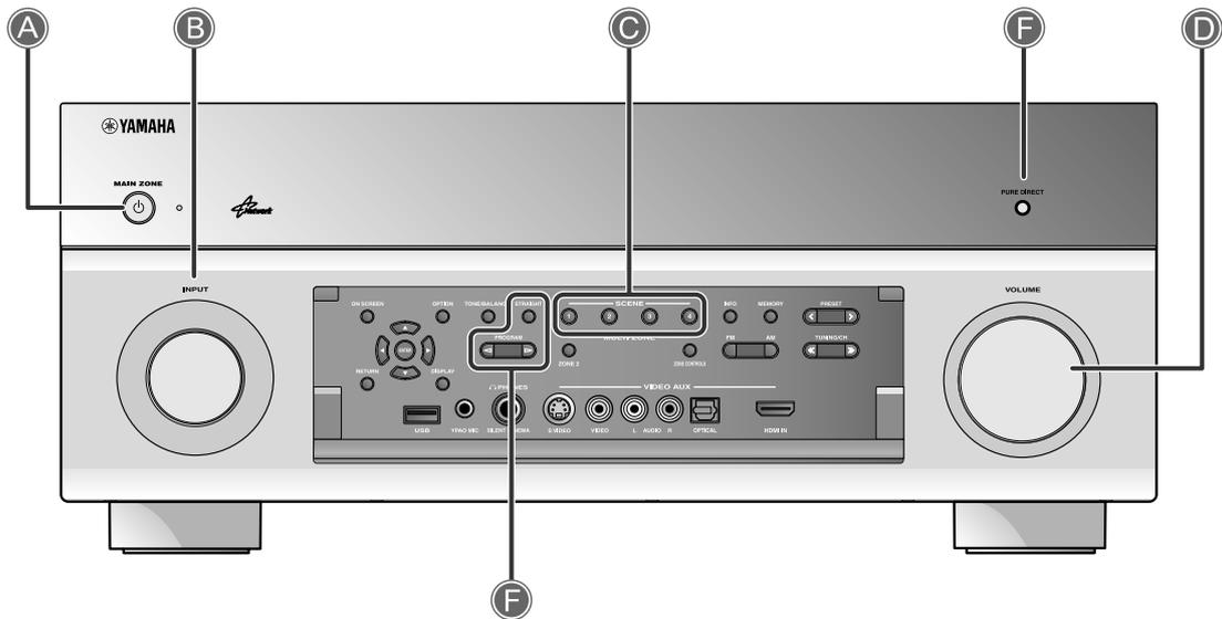
**A Switches this unit between on and standby mode**
