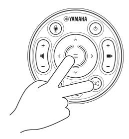
Configuration is finished after the status indicator on the front panel of the device flashes in orange five times at a 0.5-second interval.
