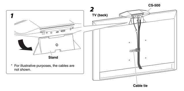
3. Adjust the camera orientation (up or down) by changing the camera's angle to the stand.
