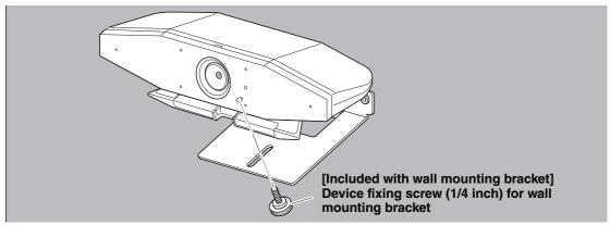
3. Adjust the camera orientation (up or down) by changing the camera's angle to the stand.
