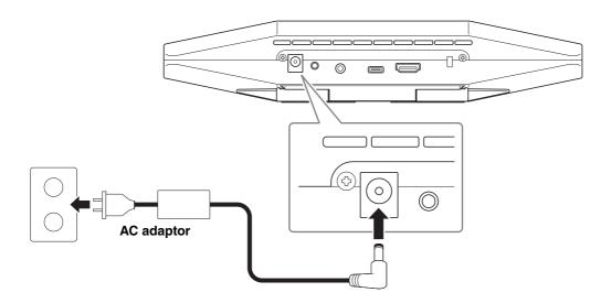
Connecting the AC adaptor automatically turns on the device.
