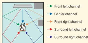
Install this unit in the corner at a 40° to 50° angle from the adjacent walls.
