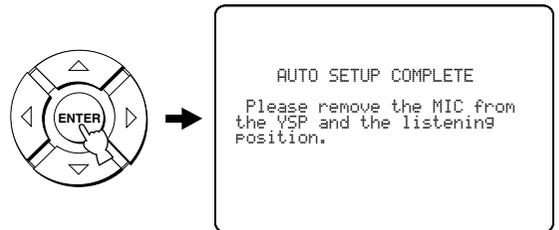
If “ENVIRONMENT CHECK [FAILED]” is displayed in step 8, the following screen is displayed after pressing ENTER. In this case, see ERROR E-1 in “Error messages for AUTO SETUP” on page 43. Press ENTER to exit AUTO SETUP and then run the procedure again from step 3.
