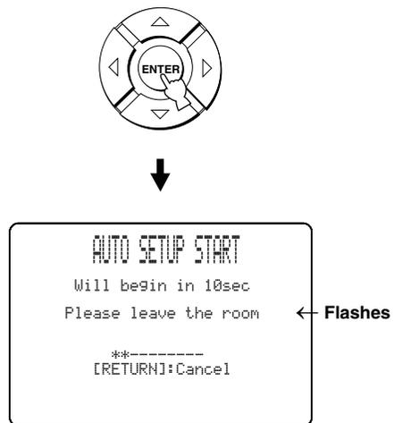
If an error occurs, an error buzzer is played and an error message is displayed. See “Error messages for AUTO SETUP” on page 43 for a complete list of error messages and their proper remedies. Follow the instructions and perform the AUTO SETUP procedure again.
