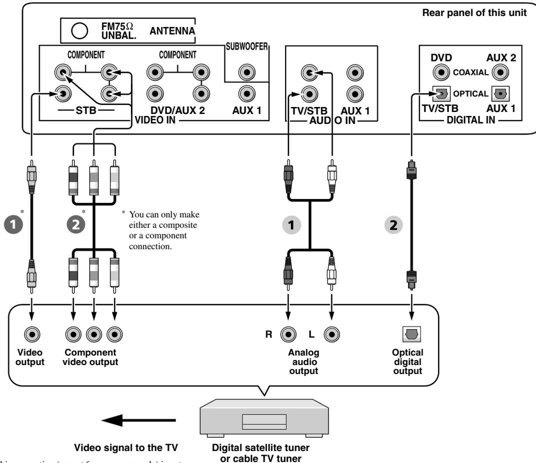
\* This connection (except for a game console) is not necessary if your TV has a built-in digital satellite tuner, cable TV tuner, or digital airwave tuner.
