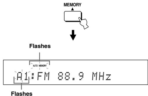
When automatic preset tuning is completed, the front panel display shows the frequency of the last preset station.
