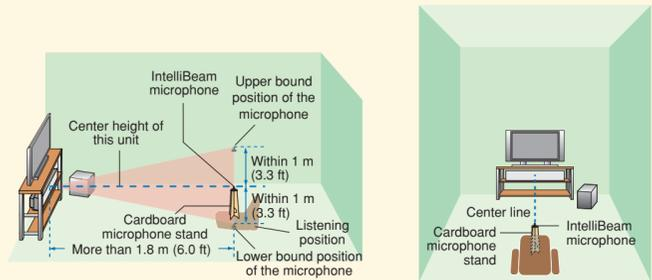
Place the IntelliBeam microphone on the extended center line of this unit and 1.8 m (6.0 ft) or more away from it. Also, make sure place the IntelliBeam microphone within 1 m (3.3 ft) upper or lower from the center height of this unit.
