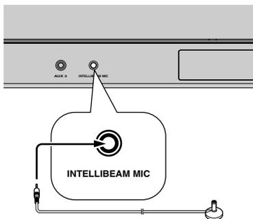
**3 Place the IntelliBeam microphone on a flat level surface more than 1.8 m (6.0 ft) from the front of the unit and within 1 m (3.3 ft) upper or lower from the center height of the unit with the IntelliBeam microphone facing upward at your normal listening position.**
