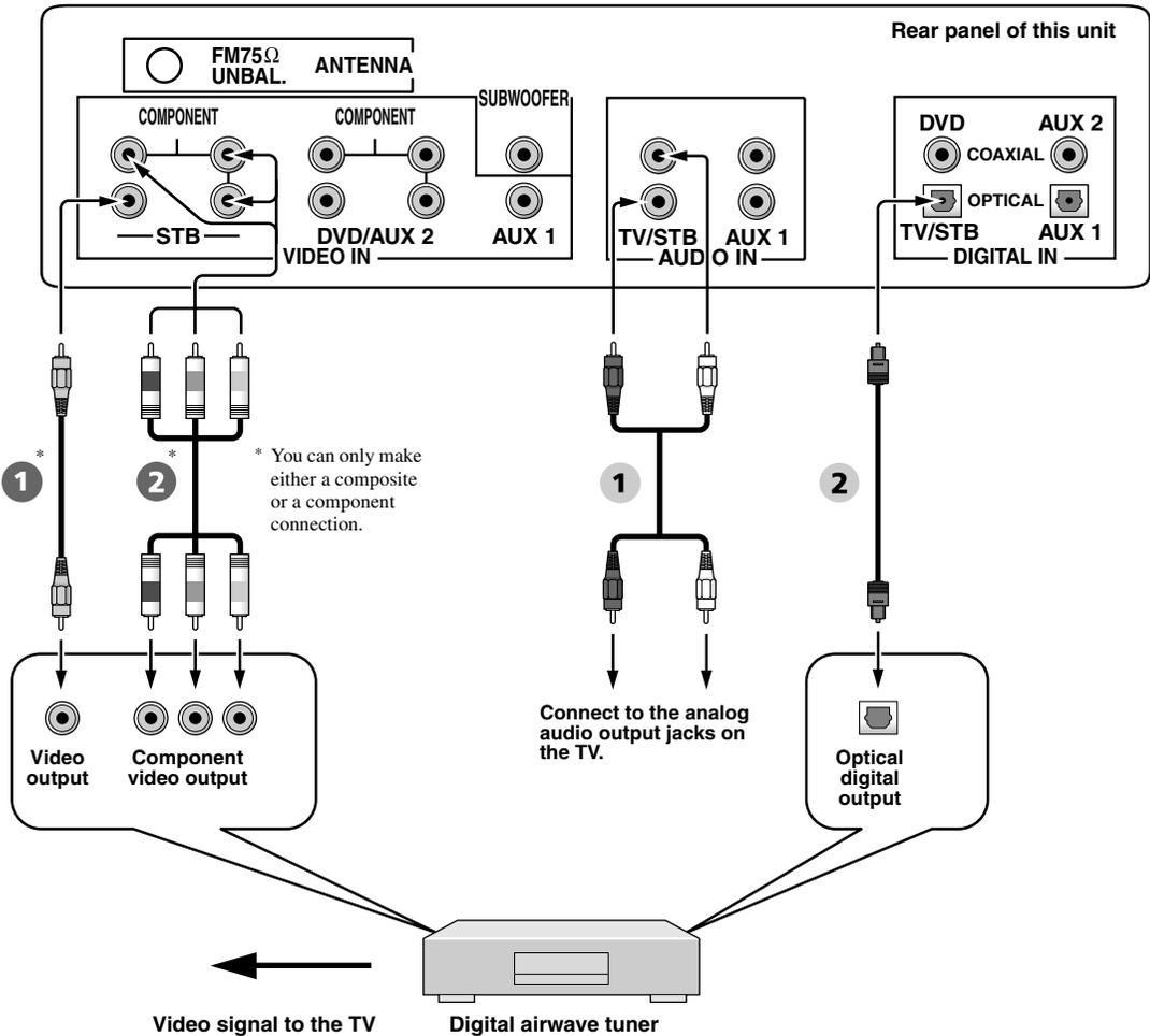
\* This connection (except for a game console) is not necessary if your TV has a built-in digital satellite tuner, cable TV tuner, or digital airwave tuner.
