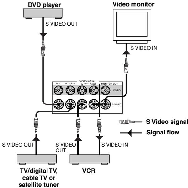
If your video component has “S” (high-resolution) video jacks, they can be connected to this unit’s S VIDEO jacks. Otherwise, connect the composite video jacks of your video component to this unit’s composite video jacks.
