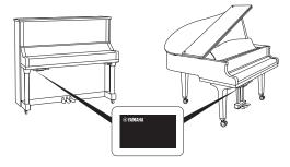
The model number can be found on or near the name plate, which is at the bottom of the control unit as shown in the illustration. Confirm the model name first since the availability of functions differs depending on the model.
