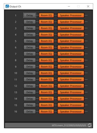
This performs the "Delay," Room EQ," and "Speaker Processor" signal processing.
