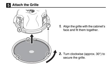
CAUTION If the grille is not sufficiently turned, it may fall off. Sufficiently turn the grille, until the fastening sections of the grille and speaker are securely engaged. • If the ceiling material is soft, the baffle surface may sink into the ceiling material due to overtightening of the attachment screws, and the grill may not fit properly.
