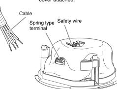
2. Insert the cable into each terminal. Insert the cable while holding the lever, and when fully inserted, release your finger from the lever to securely connect. (Lever operation is not required for solid core wire.) Make sure that the cables cannot be pulled out.
