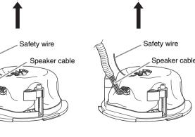
3. While lifting up the speaker, turn the screwdriver clockwise to tighten the attachment screw
