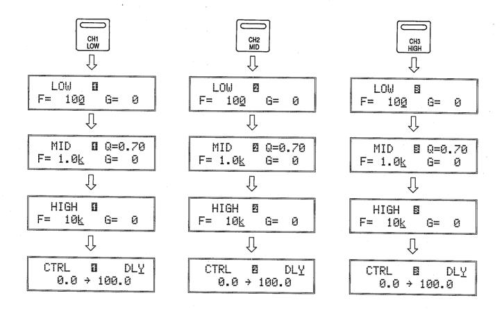
Use the  $\triangleleft$  and  $\triangleright$  CURSOR keys to move the underline cursor to the required parameter. Use the  $\triangle$  and  $\nabla$  parameter editing keys to set the value of the selected parameter.
