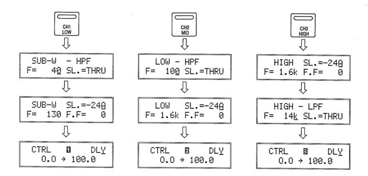
Use the  $\triangleleft$  and  $\triangleright$  CURSOR keys to move the underline cursor to the required parameter. Use the  $\triangle$  and  $\nabla$  parameter editing keys to set the value of the selected parameter.
