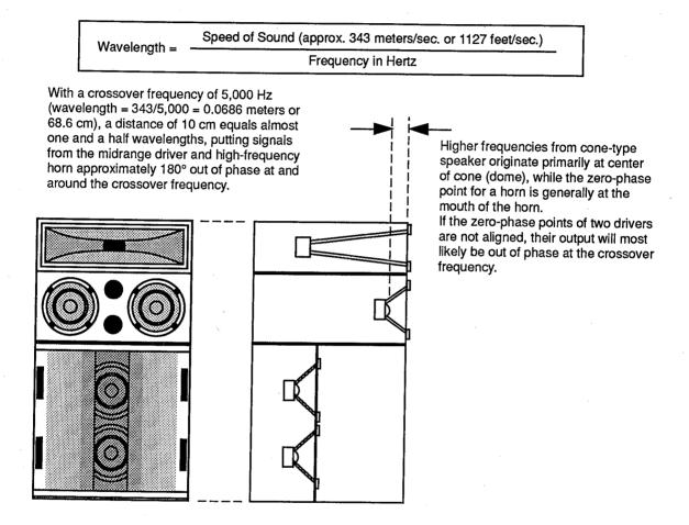
In this example, the 10-centimeter distance between the zero-phase points of the midrange drivers and high-frequency horn results in almost 180 degrees phase difference — the worst possible case. This situation can be resolved quite easily with the D1030 in its 3-way DE-LAY & CROSSOVER mode by setting the midrange (CH2) delay to about 20 milliseconds — or 68 millimeters if the display mode is set to meters. Fine adjustment is best carried out by ear.
