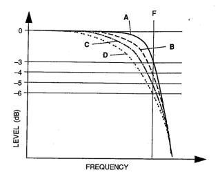
Note: The SUB-W F (frequency) parameter can be set as high as 18 kHz to allow the use of a supplemental full-range speaker system rather than a sub-woofer system.
