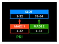
The MADI1 (Channel 1-32) signals are input to Slot 1-32, and the MADI2 (Channel 1-32) signals are input to SLOT 33-64
