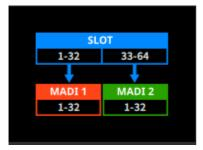
The SLOT 1-32 signals are output to MADI1 (Channel 1-32), and the Slot 33-64 signals are output to MADI2 (Channel 1-32)
