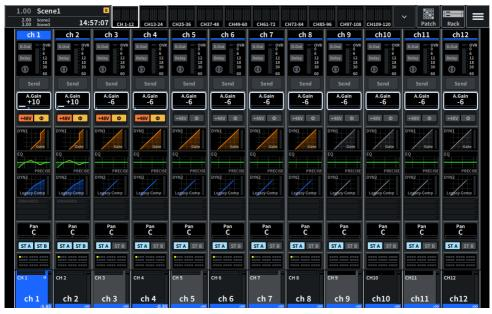
This screen simultaneously displays the main parameters of the parts of the 12 channels for which layers are selected.
